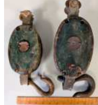
Two 19th c nautical iron & wood block & tackle pulleys Upson-Walton Co., OH
